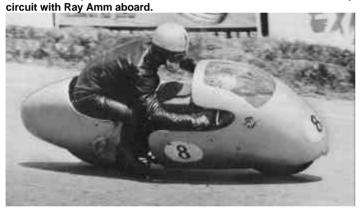
Whilst full frontal fairings were popular in all capacity classes in the 1950s. Tail fairings were rarer, generally being fitted to the 125 cc. machines, which needed all the help they could get. Slipstreaming by following competitors was rendered less effective because of the reduced wake. This is multi-world-champion Carlo Ubbiali winning the 1956 Belgian GP on a 125 cc MV Agusta.
