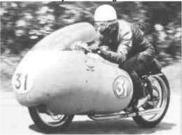
With their own full size wind tunnel the Carcano designed Moto Guzzis of the 1950s. probably had the most efficient "dushbin" fairings of the period. Shown here is a 1957 500 cc. single cylinder at the TT with Keith Campbell aboard. It's 150 mph top speed is testament to the quality of the aerodynamics.
