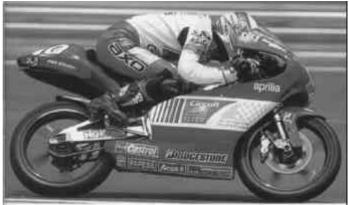
The aerodynamics of this 1999 125 cc. Aprilia is only different in detail to that of the older Honda on the left. The belly pan is narrower and fills almost completely the gap between the two wheels. Note also the front mudguard which is faired in to blend the air over the front forks. At the rear the seat back is larger to help smooth the flow as it leaves Jeronimo Vidal's back.
